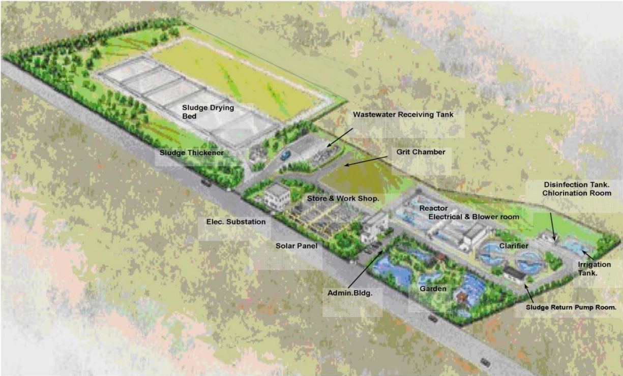
Figure (3.7): Layout of Jericho WWTP
